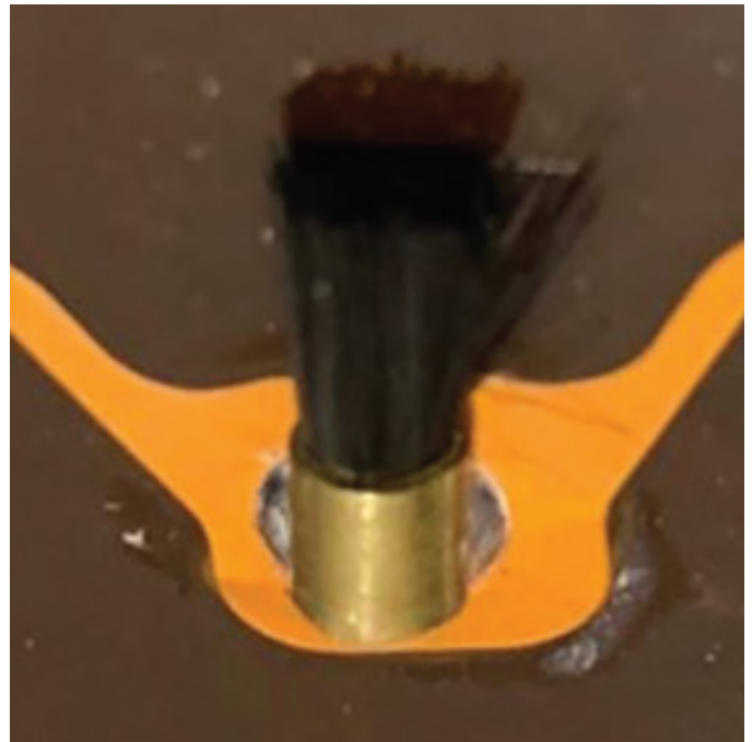
Needlepoint Electrode (0.25”) core is brass.
